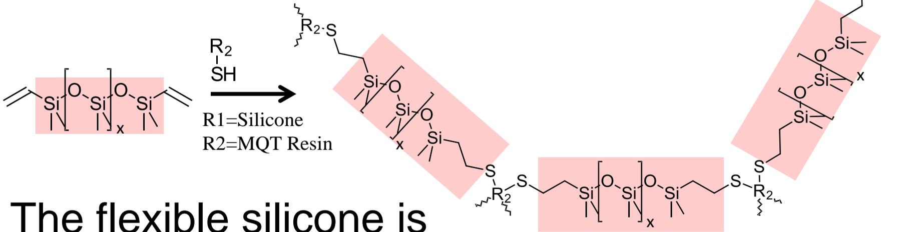
The flexible silicone is in the backbone.
