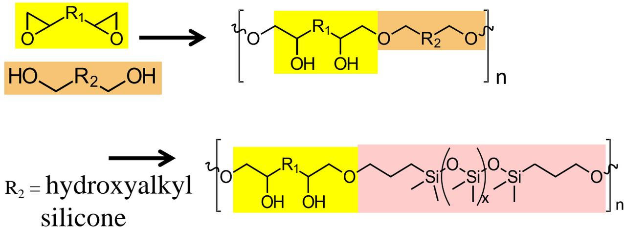
The flexible silicone is in the backbone elongation is high
